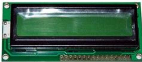
An LCD is made with either a passive matrix or an active matrix display grid. An active matrix has a transistor located at each pixel intersection, requiring less current to control the luminance of a pixel. For this reason, the current in an active matrix display can be switched on and off more frequently, improving the screen refresh time. Passive matrix LCD's have dual scanning, meaning that they scan the grid twice with current in the same
