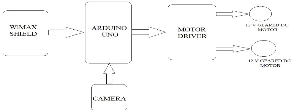
**FIG. BLOCK DIAGRAM OF ROBOTIC CAR USING WiMAX**
