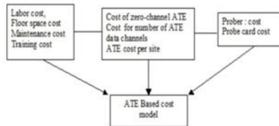
FIGURE 2: ECONOMIC COST MODEL FOR ATE BASED VLSI TESTING
