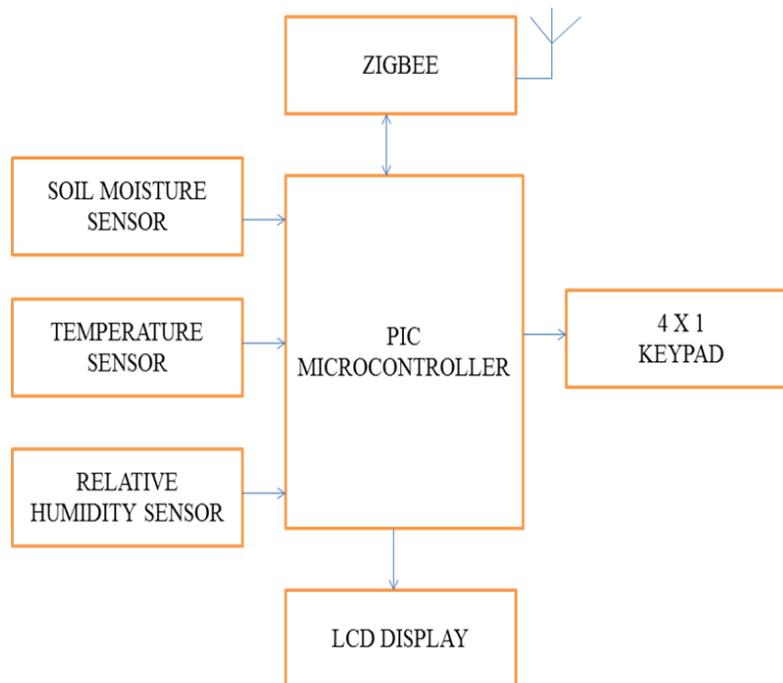
FIG. 1: BLOCK DIAGRAM OF TRANSMITTER SECTION
