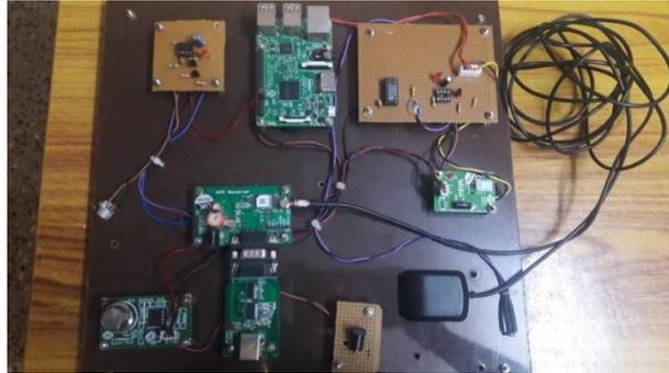
**FIGURE 7: PROPOSED AIR AND NOISE MONITORING SYSTEM**
