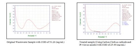
FIGURE 2. DIFFERENT PULSE VOLUMERIC (DPV) RESULTS
