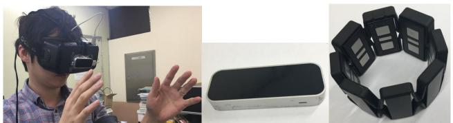
Fig. 1: Hardware Configuration of our system (left: Hmd with Myo, center: Leap Motion, right: Myo)
