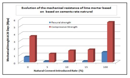
FIGURE1: MECHANICAL CHARACTERISTICS OF ELABORATE MORTARS
