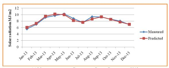
(B) MEASURED VERSUS PREDICTED SOLAR RADIATION-2013 MODEL 4
