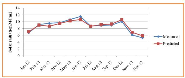
(A) MEASURED VERSUS PREDICTED SOLAR RADIATION-2012 MODEL 5
