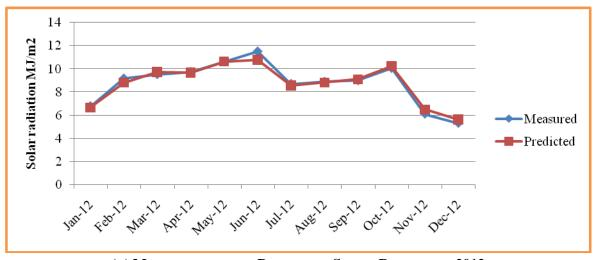
(a) Measured versus Predicted Solar Radiation-2012 Model 2
