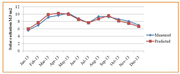
(B) MEASURED VERSUS PREDICTED SOLAR RADIATION-2013 MODEL 2
