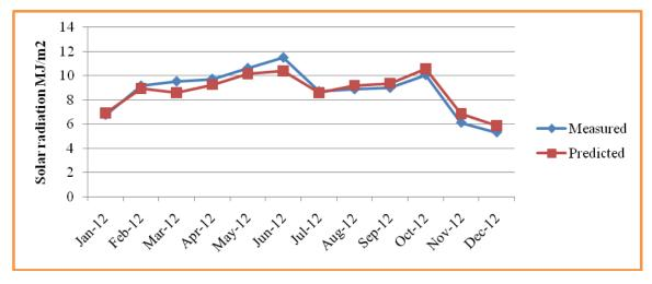
(A) MEASURED VERSUS PREDICTED SOLAR RADIATION-2012 MODEL 4
