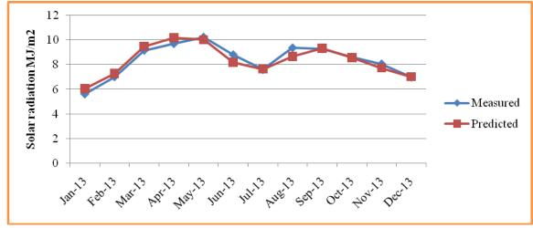
(B) MEASURED VERSUS PREDICTED SOLAR RADIATION-2013 MODEL 3
