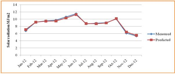
(A) MEASURED VERSUS PREDICTED SOLAR RADIATION-2012 MODEL 1
