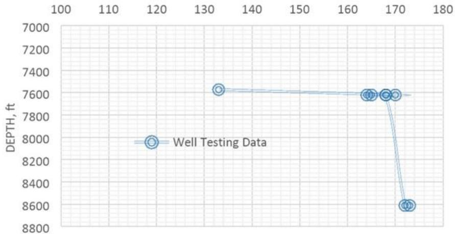
**FIGURE 4: TEMPERATURE PROFILE REVERSAL AT BOTTOM OF WELL #12 IN BLOCK 276 P1-SAND**
