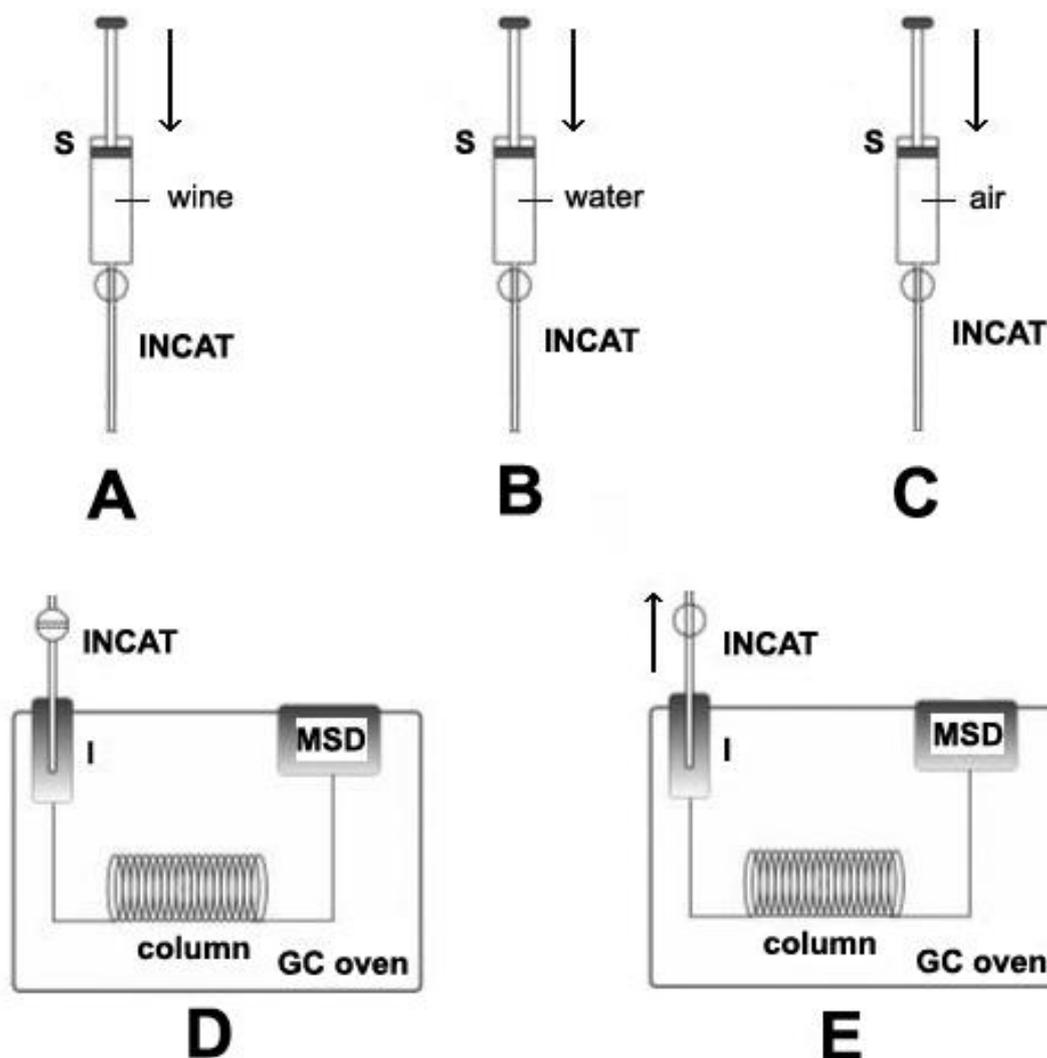
**FIGURE 2 SCHEME OF SORPTION AND DESORPTION PROCESS OF INCAT DEVICE. A – SAMPLING OF WINE SAMPLES, B – FLUSHING OF INCAT DEVICE BY WATER TO REMOVE RESIDUAL WINE AND WET ALUMINA, C – REMOVING OF RESIDUAL WATER, D – DESORPTION, E – CLEANING. S - SYRINGE; MSD – MASS SPECTROMETRIC DETECTOR; I - INJECTOR.**
