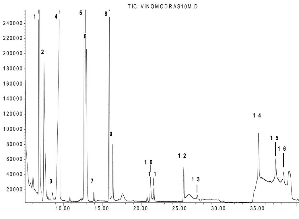
**FIGURE 3. GC-MS/SIM CHROMATOGRAM OF A WHITE WINE AT SAMPLING VOLUME 100 ML USING INCAT DEVICE. (1) ethylacetate; (2) i-butanol; (3) formic acid; (4) acetic acid; (5) i-amylalcohol; (6) 1-butanol-2-methyl; (7) propyleneglycol; (8) 2,3-butanediol; (9) 1,3-butanediol; (10) i-amylacetate; (11) butyrolactone; (12) succinic anhydrid; (13) hexanoic acid; (14) 2-phenylethylalcohol; (15) ethylhydrogensuccinate; (16) octanoic acid.**
