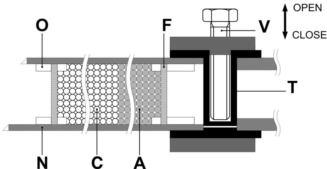
**FIGURE 1 SCHEME OF INCAT SYSTEM [17, 18]. (N) STAINLESS STEEL NEEDLE; (O) STAINLESS STEEL O-RING; (F) STAINLESS STEEL FRITS; (C) ADSORBENT CARBOXEN 1000; (A) ADSORBENT ALUMINA; (V) SHUT-OFF MICRO VALVE WITH STAINLESS STEEL BODY; AND (T) VITON TUBING.**
