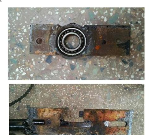
The main function of the bearing is to prevent sliding friction between two parts. Here ball bearing is used with ISO standard 6001. The inner diameter where the bearing casing is fix is 15mm and outer diameter is 30mm. It is also called as pedestal or bearing housing. The second fabricated part in which bearing housing is attached is fixed on both side of rear wheel of the cycle.
