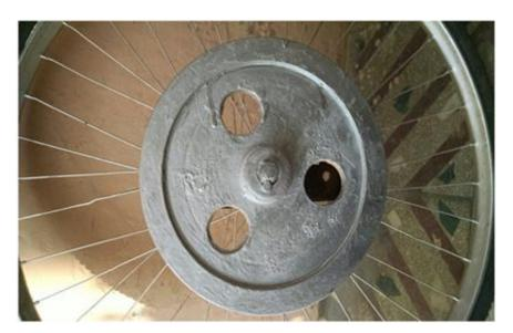
The bicycle consists of one small pulley and one big pulley. The big pulley is connected on other side of the rear wheel which is inserted into center shaft. The small pulley is attached to pump which is placed in carrier of cycle and both pulley is connected by means of belt. The Big pulley and small pulley ratio is 1:3. When big pulley completes its one rotation, the small pulley completes its three rotation. And water is lifted its required height.
