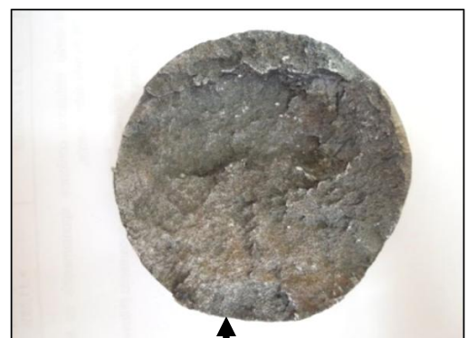
FIGURE 6. IMAGE OF THE FRACTURE SURFACE OF THE UNDERSIDE OF FRACTURED KING PIN. THE ARROW SHOWS THE FRACTURE ORIGIN.
