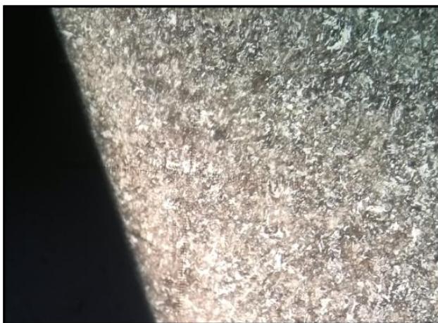
FIGURE 2. OPTICAL MICROSCOPE IMAGE OF THE KINGPIN STEEL MICROSTRUCTURE SHOWING TEMPERED MARTENSITE AND BAINITE. ETCHANT: NITAL 3%.
