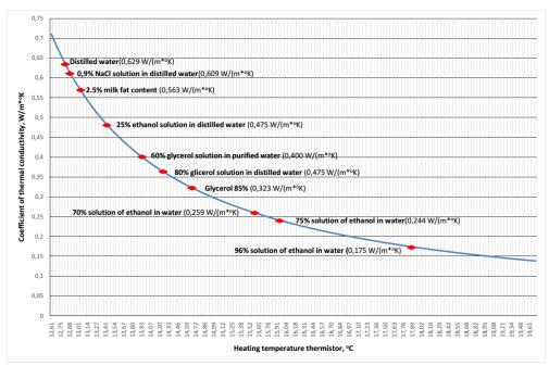
Fig. 5 Graph of the thermal conductivity of liquids experimental heating temperature thermistor according to measurements at the research sample of +40  $^{\circ}$ C
