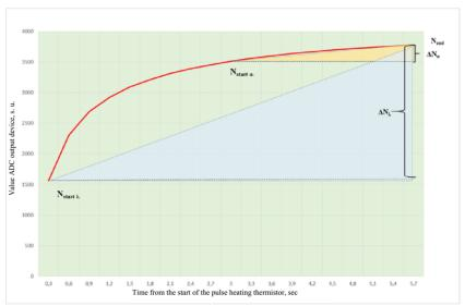
FIG. 4 HEATING THERMOGRAM OF THERMISTOR
