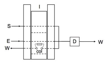
FIGURE 2. FLOW DIAGRAM OF THE SYSTEM FOR 5,5<sup>-</sup>-DI determination. I: sliding-bar injector, S: sample (2.4 mL min<sup>-1</sup>), E: eluent (3.0 mL min<sup>-1</sup>), col: mini-column (2-mm diameter, 15-mm long, filled with green coconut fiber), D: spectrophotometer (612 nm) and W: waste.
