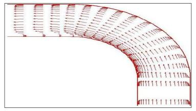
FIGURE 4. FLOW FIELD VELOCITY VECTOR DISTRIBUTION
