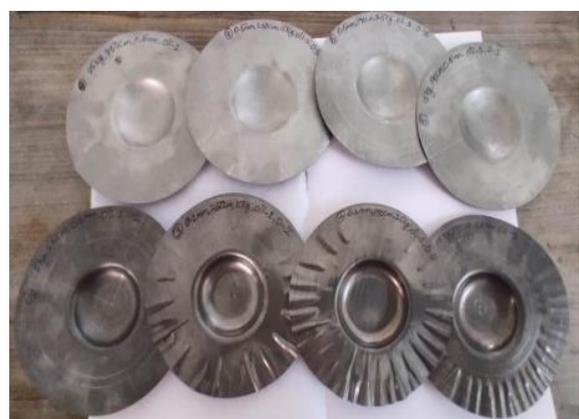
**FIGURE 3: Deformed Superni 718work pieces**
