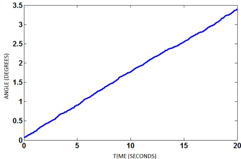
**FIGURE 9. CUMULATIVE ERROR POSITION CALCULATION WITH GYROSCOPE**
