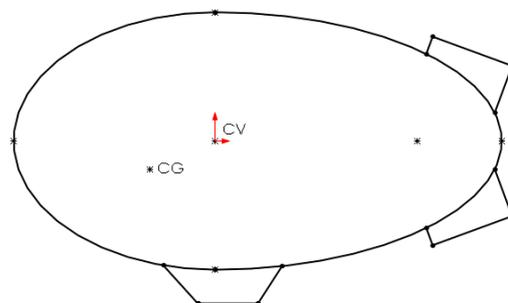
**FIGURE 3. CENTER OF GRAVITY AND CENTER OF VOLUME OF A DIRIGIBLE.**
