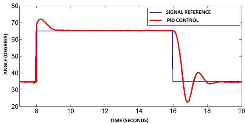
**FIGURE 12. RESPONSE TURNING SYSTEM CONTROLLED BY PID ABOUT 30°**
