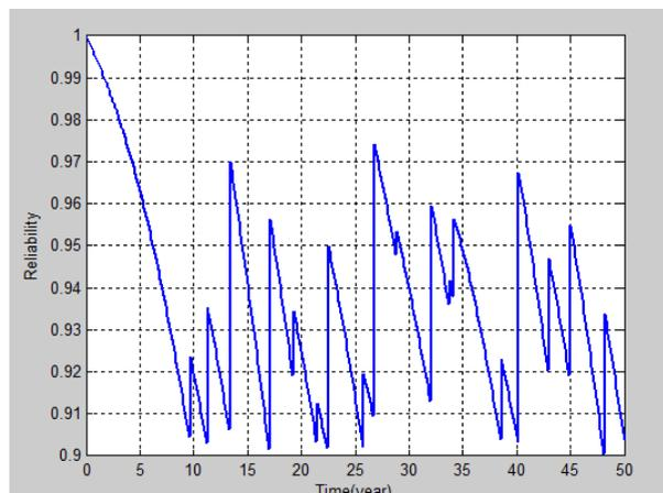
**FIGURE 3. RELIABILITY CURVE ( $T_M = 50$  years,  $R_s(t) \geq 0.9$ )**
