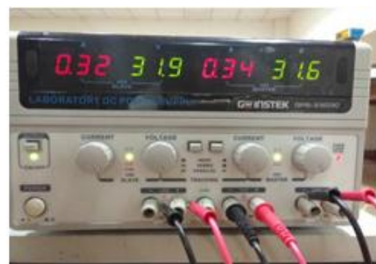
FIGURE 3: GUWEI DC POWER SUPPLY
