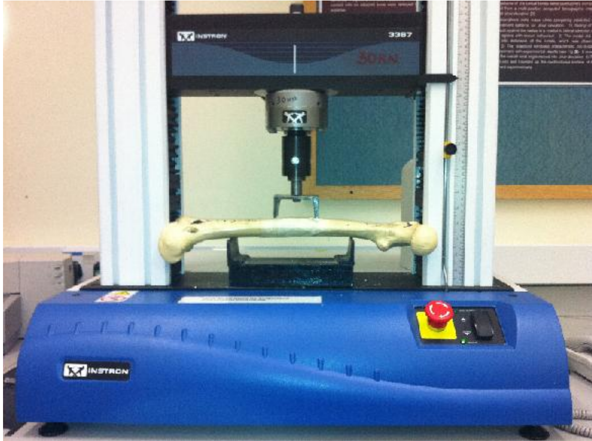
FIGURE 2: SHOWING FOUR POINT TESTING IN AP PLANE
