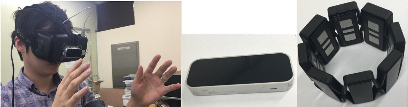
**Fig. 1: Hardware Configuration of our system (left: Hmd with Myo, center: Leap Motion, right: Myo)**
