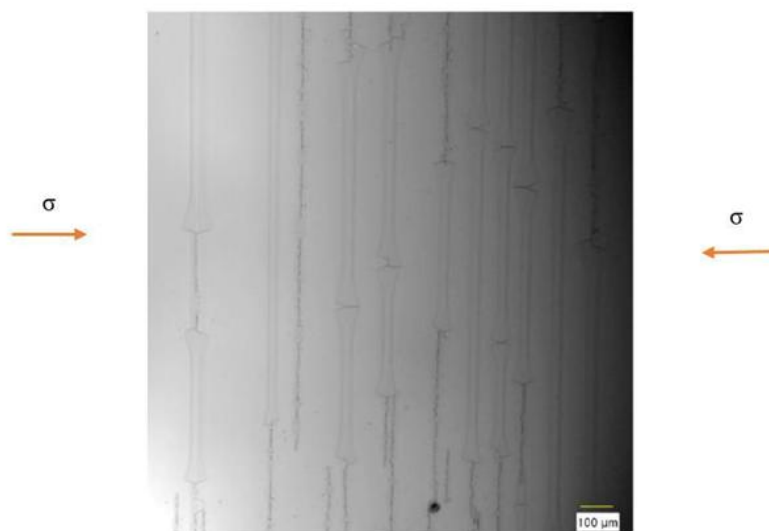
FIG. 6. Optical Microscope observation of buckles and cracks after micro-compression tests. Concomitance of buckles and cracks (x 5). Buckles and transverse cracks (x 20).
