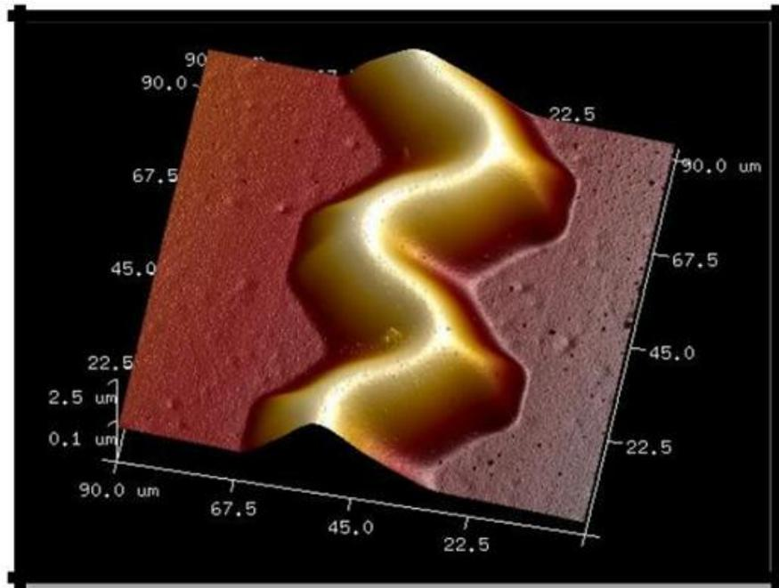
**FIG. 7. Telephone cord morphology observed during relaxation of compressive stress, obtained by AFM**
