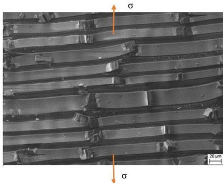
**FIG. 4. Scanning Electron Micrograph of fractured tensile specimen**
