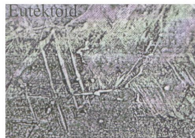
FIGURE 8. MICROSTRUCTURE OF ALLOY QUENCHED FROM 900 °C AND AGED AT 400 °C FOR 1h (x960)
