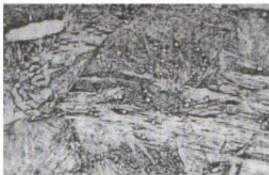
FIGURE 5. MICROSTRUCTURE OF ALLOY, ANNEALED AT 850 °C FOR 10 MIN AND WATER QUENCHED (x960)
