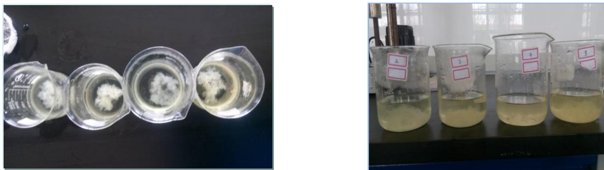
FIG. 5 SAMPLE PICTURES OF FRACTURE LIQUID AFTER BREAKING WITH DIFFERENT AMMONIUM PERSULPHATE LOADING OF 0.02 wt%, 0.03wt%, 0.04wt% and 0.05wt%, RESPECTIVELY.
