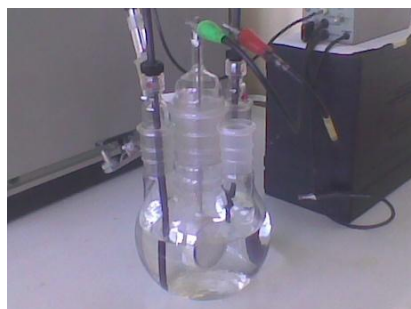
FIGURE 1. GLASS CELL FOR MEASURING CORROSION RATE
