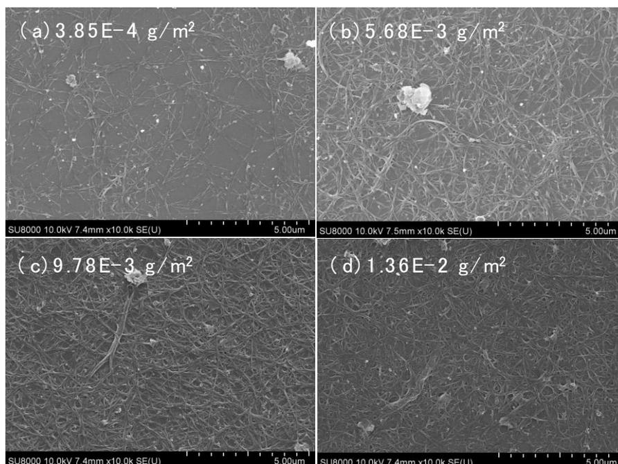
**FIG. 2: Schematic of definition of weight density (top) and SEM images of surface of thin films containing HC-SWCNTs at controlled weight densities (bottom). (a)  $3.85 \times 10^{-4} \text{ g/m}^2$ , (b)  $5.68 \times 10^{-3} \text{ g/m}^2$ , (c)  $9.78 \times 10^{-3} \text{ g/m}^2$ , and (d)  $1.36 \times 10^{-2} \text{ g/m}^2$ .**
