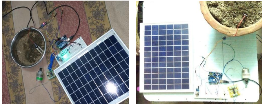
FIG 11. SNAPSHOTS OF AUTOMATIC SOIL MOISTURE MONITORING SYSTEM
