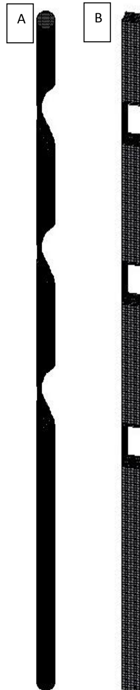
FIGURE 2. 3D DIMENSION OF HOSES THAT ARE PUSHED BY ROLLER. (A): REALIZATION MODEL, (B): SIMPLIFICATION MODEL
