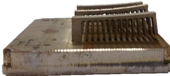
**FIGURE 3: SUPPORT CUTTING FORM THE BASE PLATE BY EDM AND RESULTING DISTORTION**
