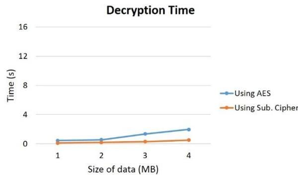
**FIGURE 2. Decryption time when AES and substitution ciphers are used**
