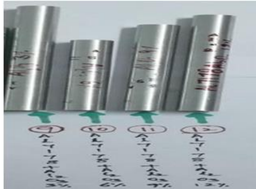
FIGURE 3: Machined Al7178 MMC's
