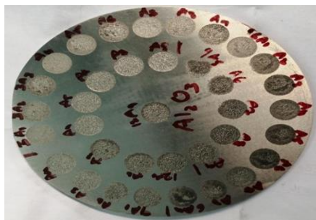
FIGURE 6: Experimentation on Superni90 work material with Aluminium and Al 2 O 3 3%, 6%, 9%, 12% as Electrodes on EDM
