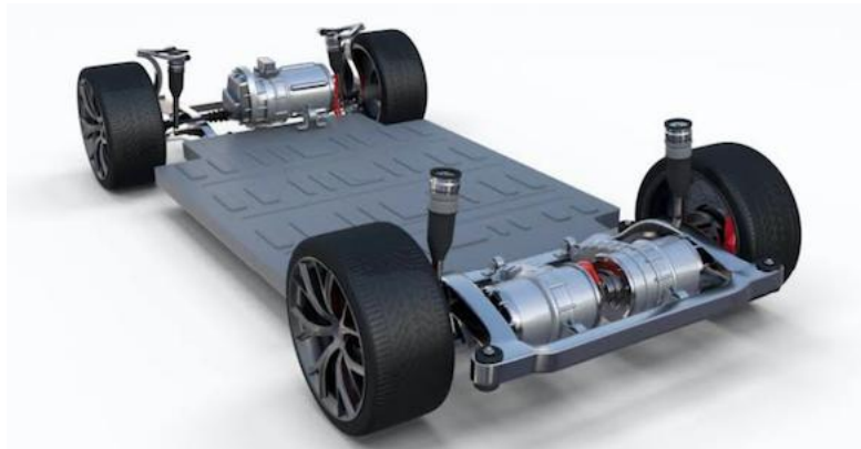
FIGURE 2: Motors incorporated in Tesla Roadster
