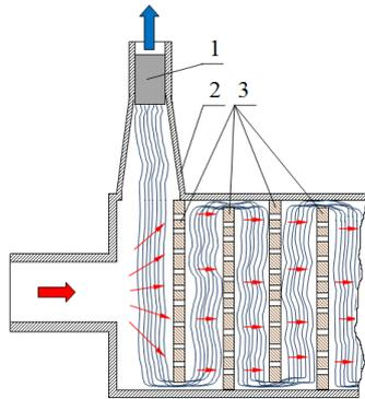
**FIGURE 1: A cross-section of the square-shaped exchanger**
