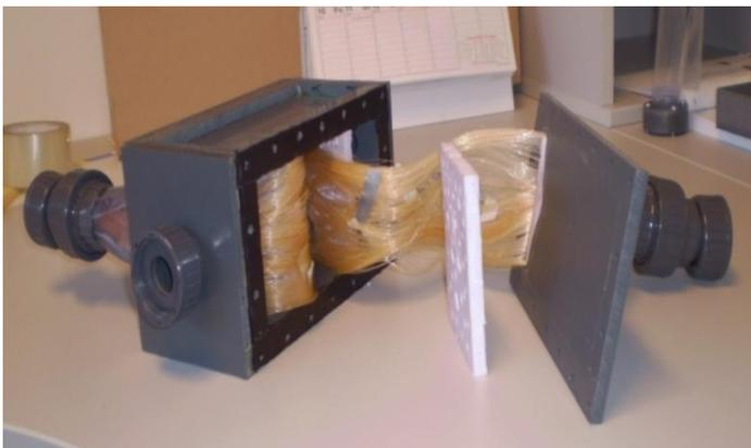
**FIGURE 3: Procedure of installing fibres and partition plates**
