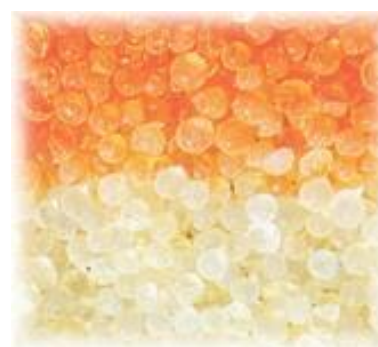
c) Type Orange gel – indicator grains
