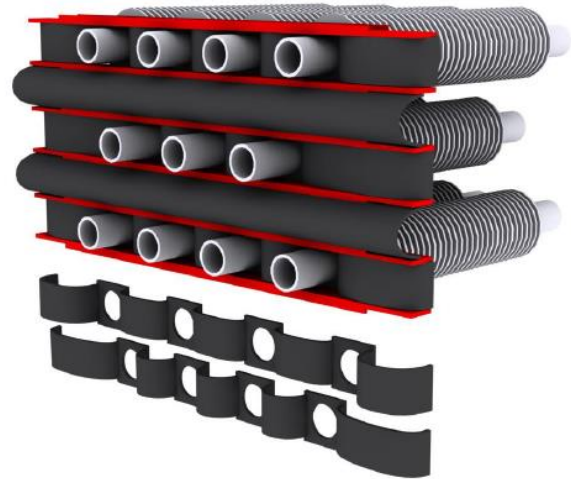
FIGURE 8: Rubber seals on the inlet side of the exchanger
