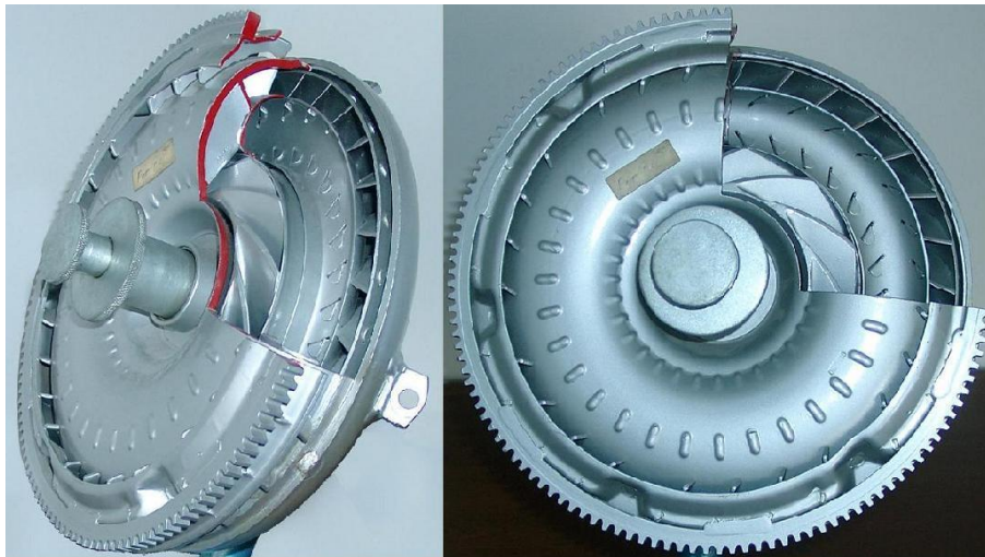
FIGURE 1 VIEW OF THE MODEL W240 AUTOMOTIVE HYDRAULIC TORQUE CONVERTER FABRICATED BY SACHS SHOWING THE EXIT OF THE TURBINE BLADING ON THE OUTER DIAMETER AND THE GUIDE VANE WHEEL DIRECTING THE FLOW FROM TURBINE TO PUMP NEAR THE HUB
