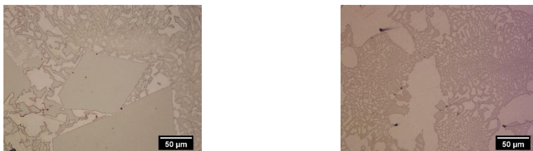
FIG. 1. OPTICAL MICROGRAPHS SHOWING MICROSTRUCTURES OBTAINED AFTER THE BRAZING CYCLE FOR BATCH A (LEFT) AND BATCH B (RIGHT)
