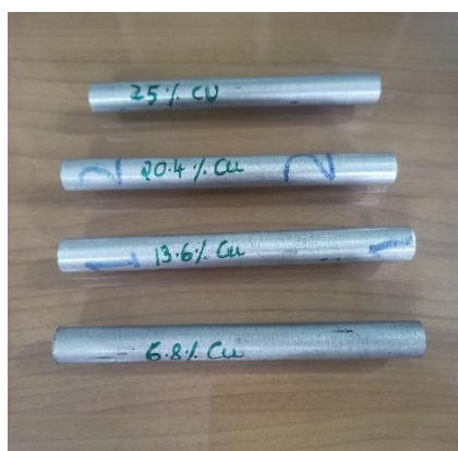
FIGURE 2: Al2021 Electrodes with varying % of Cu
