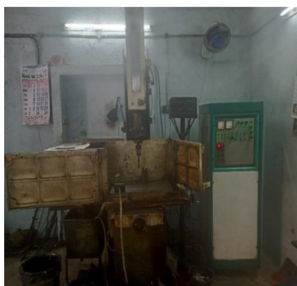
FIGURE 1: Die-sinking EDM machine
