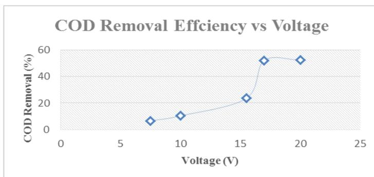
**FIGURE 3. EFFECT OF VOLTAGE ON COD REMOVAL EFFICIENCY**
