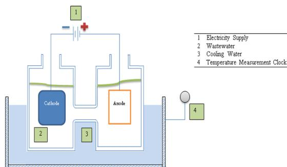
**FIGURE 1. ELECTRO COAGULATION EXPERIMENTAL SYSTEM**
