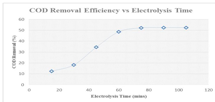
**FIGURE 4. EFFECT OF ELECTROLYSIS TIME ON COD REMOVAL EFFICIENCY**
