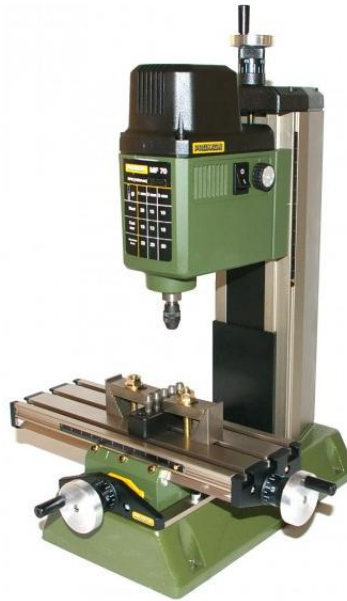
FIG. 1 WORKBENCH TYPE DRILLING MACHINE TOOL (PROXXON MF70)
