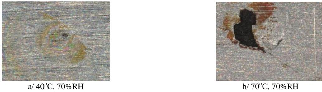
**FIGURE 4. The appearance of the as-received flat samples with saturated MgCl<sub>2</sub> droplets after 30 days, (160x)**
