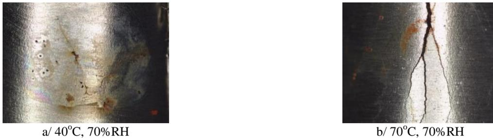
**FIGURE 15.**The appearance of the sensitized U-bend samples with saturated solution of  $MgCl_2$  droplets (12x)
