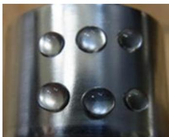
**FIGURE 2.U-bend specimen with freshly deposited droplets**
