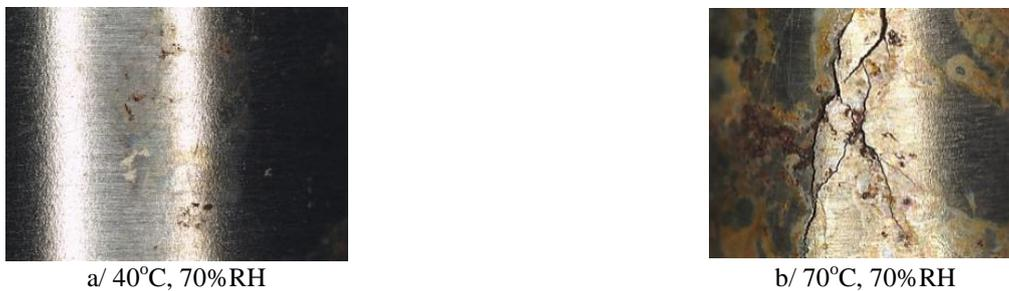
**FIGURE 13.**The appearance of the sensitized U-bend samples with saturated solution of NaCl droplets (12x)
