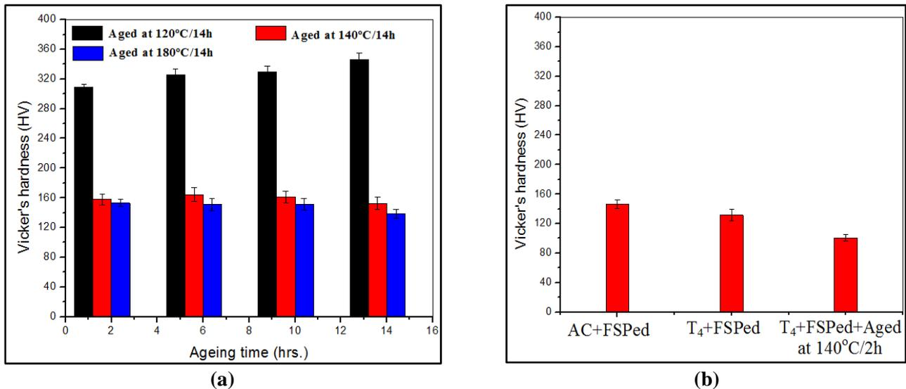
**FIGURE 8: The Vicker's hardness bar diagrams are exhibited hardening effect at different conditions: (a) after different ageing treatments, and (b) after different FSPed conditions. (1000 rpm and 70 mm/min)**
