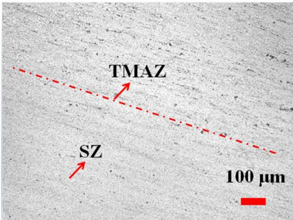
**FIGURE 2: Optical micrograph of 7075 Al alloy at T<sub>4</sub>+FSPed+Post-aged at 140°C for 2h condition. (1000 rpm and 70 mm/min)**
