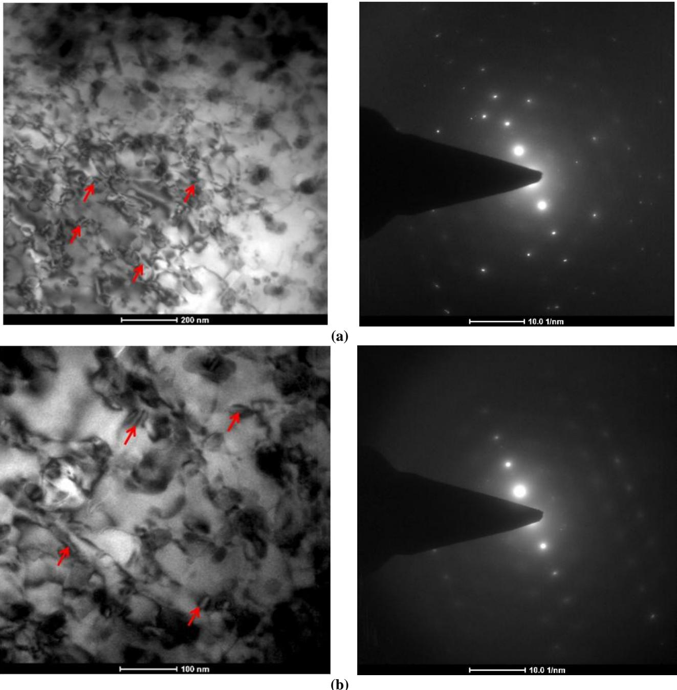
**FIGURE 5: TEM micrographs with SAD patterns of 7075 Al alloy aged at 140°C for 6h ( $T_6$ ): (a) at low magnification (200 nm), (b) at high magnification (100 nm).**
