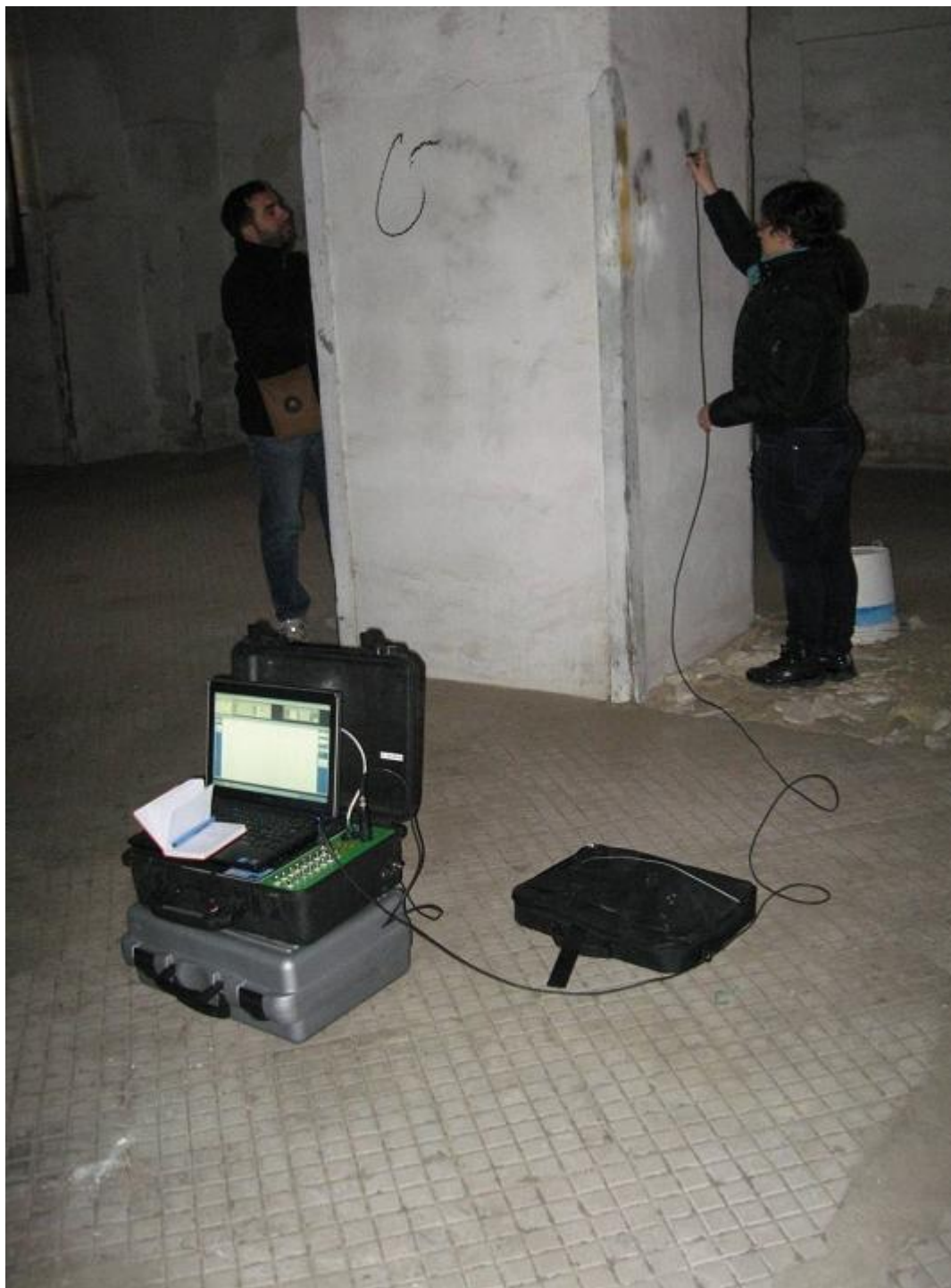
FIG. 10: IN SITU ULTRASONIC WAVE VELOCITY ACQUISITION ON PIETRA LECCESE PILLAR
