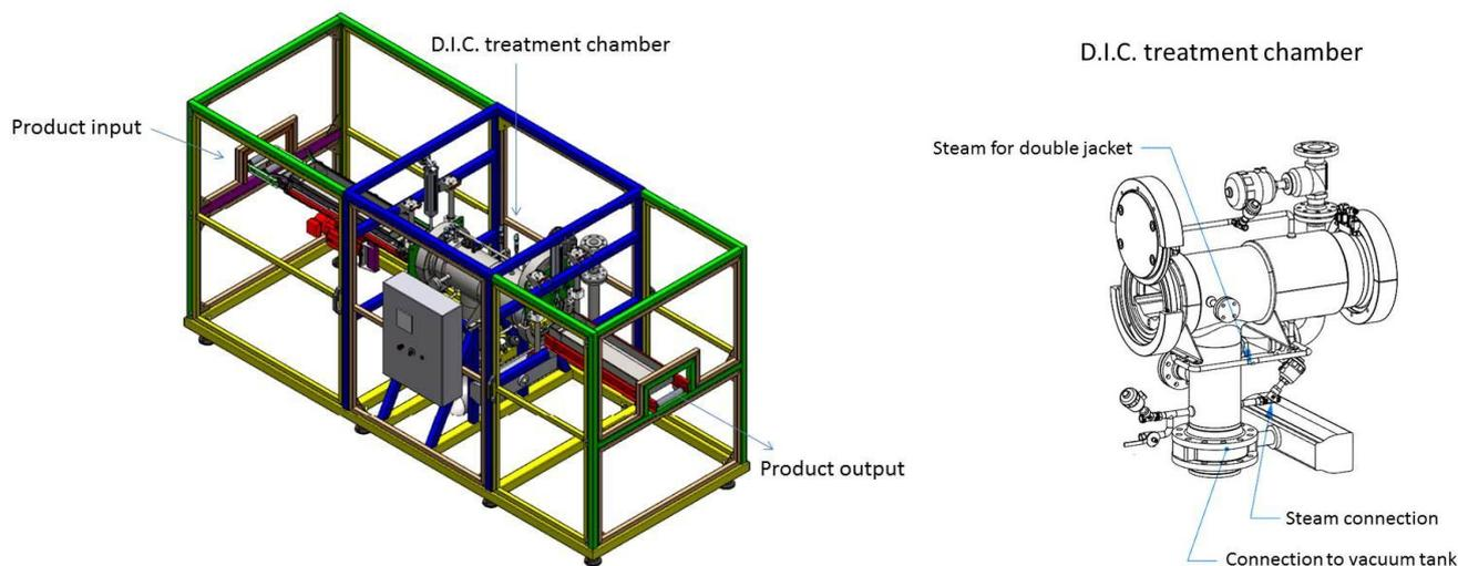
**FIGURE 1: SCHEMATIC DIAGRAM OF THE INDUSTRIAL REACTOR DICL0.3-1.0 FOR TREATMENT PER BATCH BUT SEMI-CONTINUOUS FLOW: 30L OF TREATMENT CHAMBER; AUTOMATIC INPUT AND OUTPUT OF THE PRODUCT. TREATMENT OF ABOUT 500 KG/H. OF RAPESEED, JATROPHA SEEDS, CAMELINA AND DATE SEEDS**
