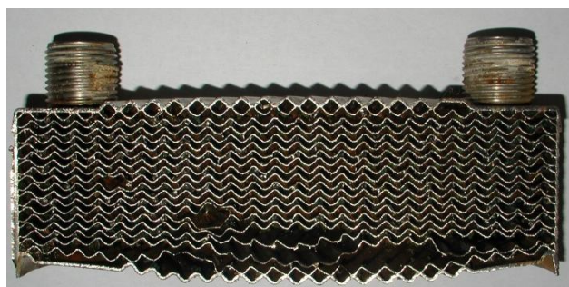
FIGURE 2: Deformation of the soldered joints of boards
