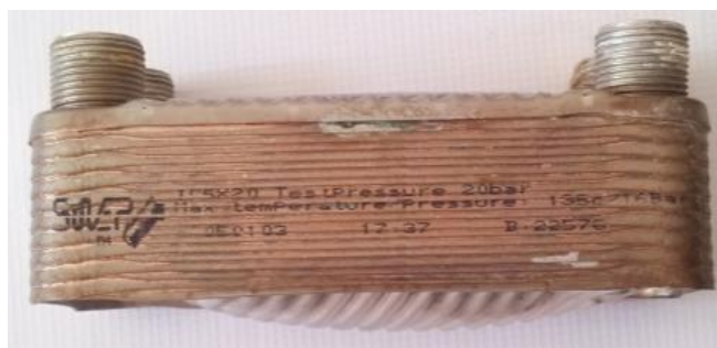
FIGURE 1: Deformation of the outer wall of the exchanger
