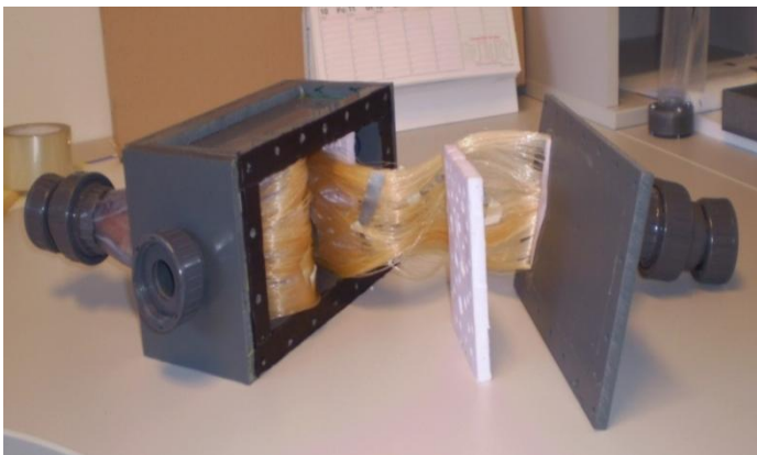
FIGURE 3: Procedure of installing fibres and partition plates
