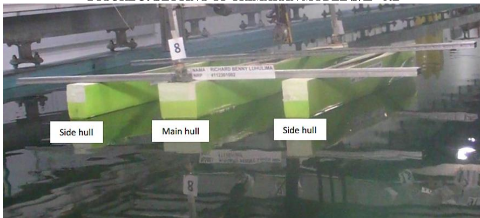
FIGURE 4. SETTING OF TRIMARAN MODEL S/L=0.3
