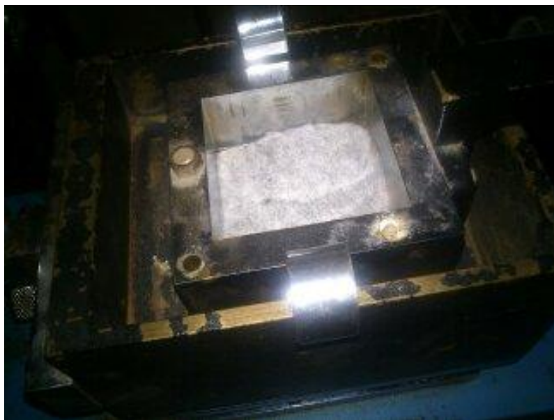
FIG.4: GEOTEXTILE PLACED IN SHEAR BOX
