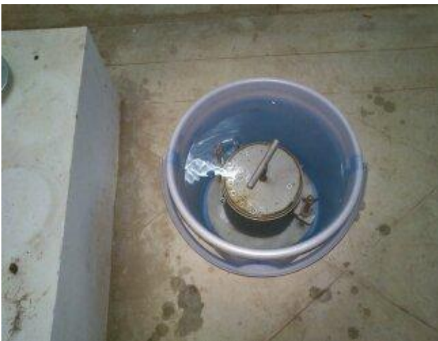
FIG.2. MOULD IS PLACED ON WATER
