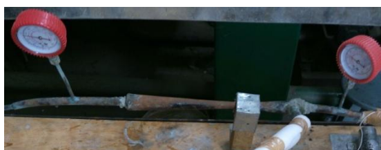
Fig.1 Illustrates the pressure variation along the ejector.
