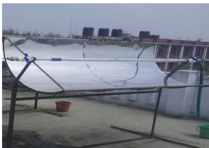
FIG 1: EXPERIMENTAL SETUP OF PTC
